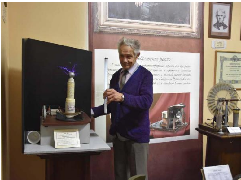
Above: Museum curator demonstrating a Tesla high voltage resonance transformer.
